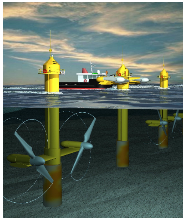
Artist's impression of maintaining a twin rotor tidal turbine.
